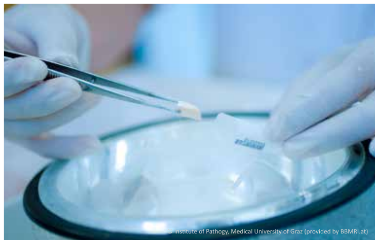
Snap-freezing of tissue samples in Isopentane pre-cooled liquid nitrogen is one of the best methods of tissue conservation for molecular analysis
